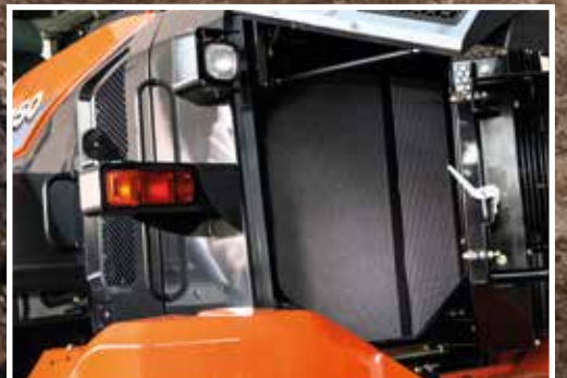
Optional anti-clogging radiators enhance durability.
