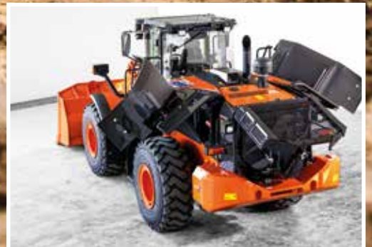
Easy access for maintenance from ground level.
